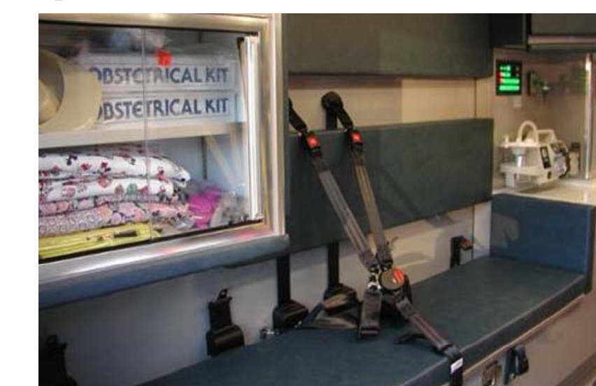
Fig. 2. Hazardous restraint configuration and head impact zone
